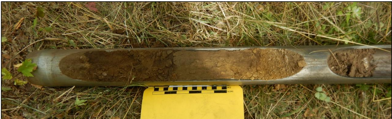
Figure 10-5: Oxidized Tailings Recovered by Percussion Drill on North Perimeter Embankment Cell #2
