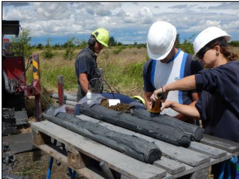
Figure 11-8: Collection of Moisture and Magnetic Susceptibility Data in the Field
