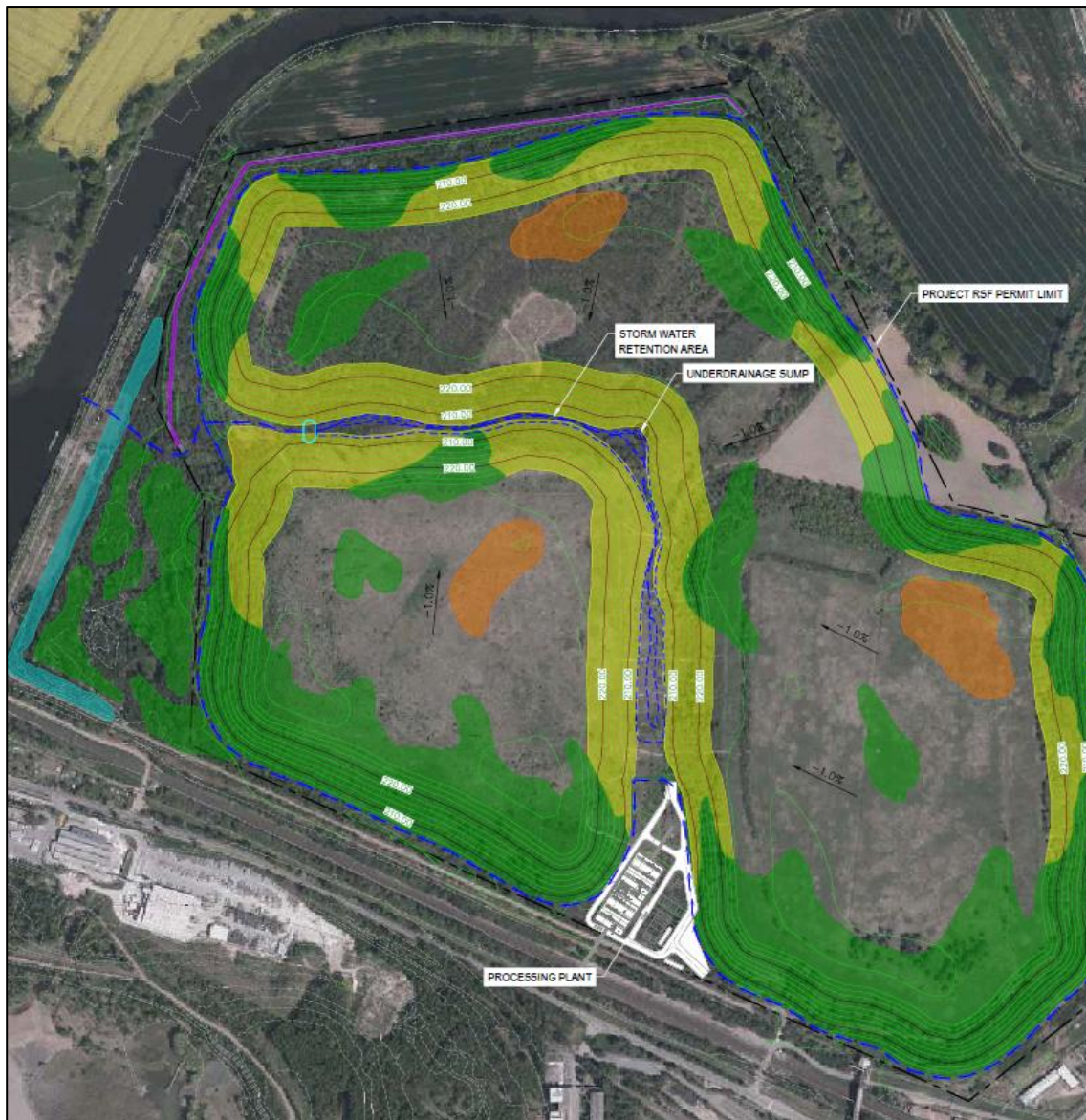
Figure 18-13: Residue Storage Facility Design – Final Landform
