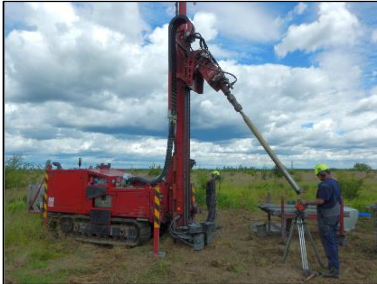
Figure 10-2: Showing Eikelkamp SonicSampDrill B.V. and Drill Crew
