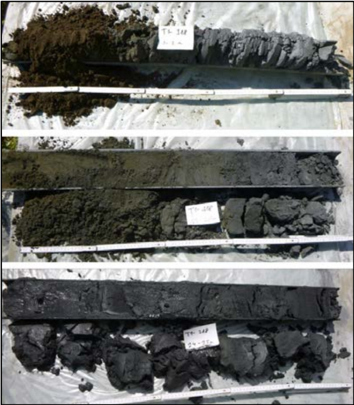
Figure 11-3: Core Photos from Drill Hole T1-318, from Depths 1-2 m, 19-20 m, and 24-25 m
