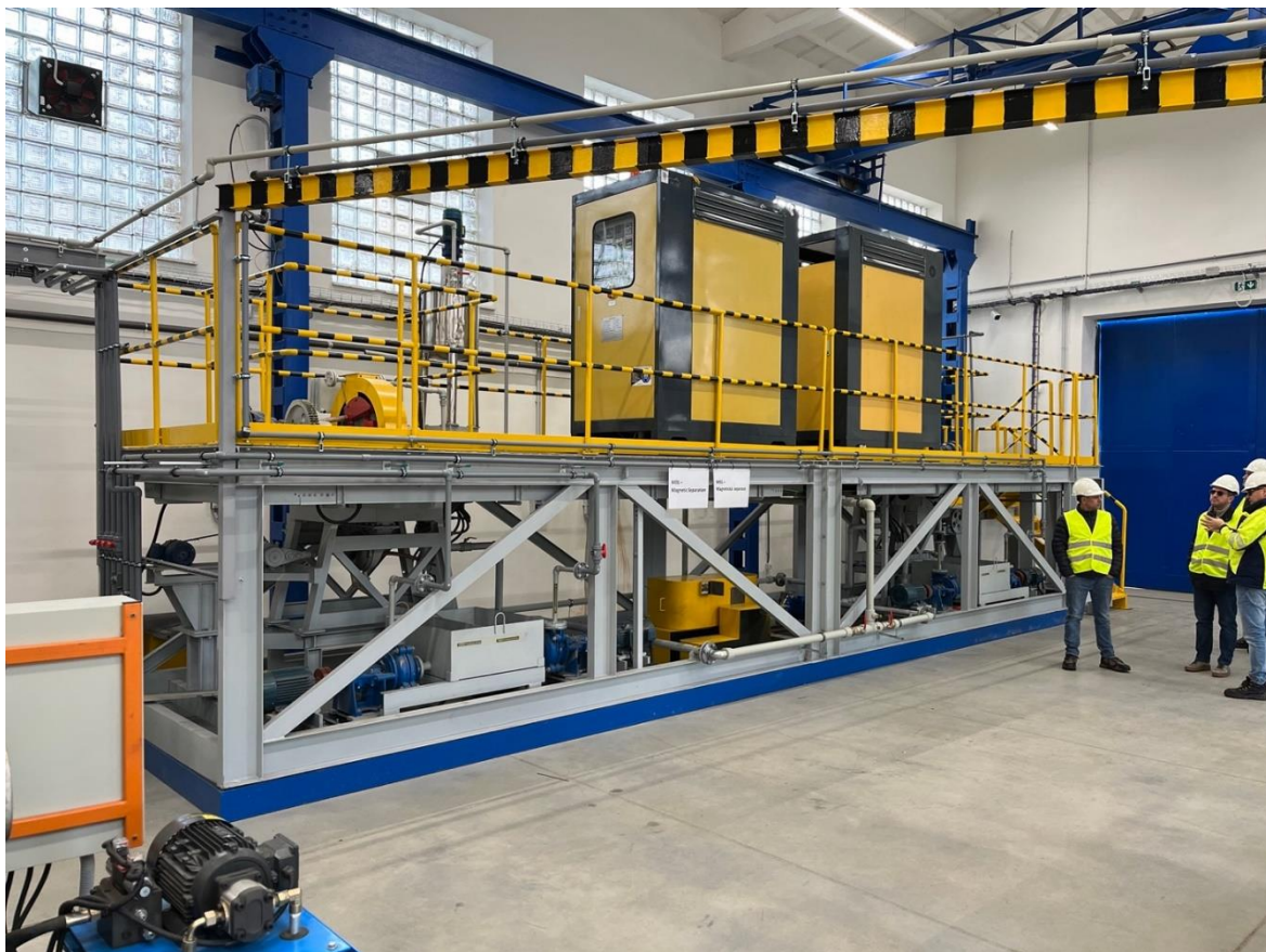
Magnetic Separation Module of the Chvaltice Manganese Project Demonstration Plant
