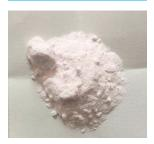
HPMSS is dried and crystallized to produce high-purity manganese sulphate monohydrate powder (HPMSM).
